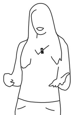
The Microphone DM05 is a microphone for closer range. It works best within approx. 12 inches (30 cm).
